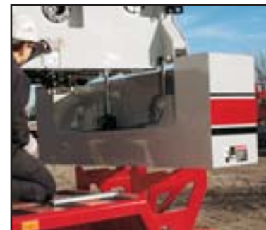
Fast & efficient hydraulic counterweight removal enhances roadability
