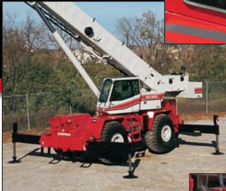
Fast & efficient hydraulic counterweight removal enhances roadability
